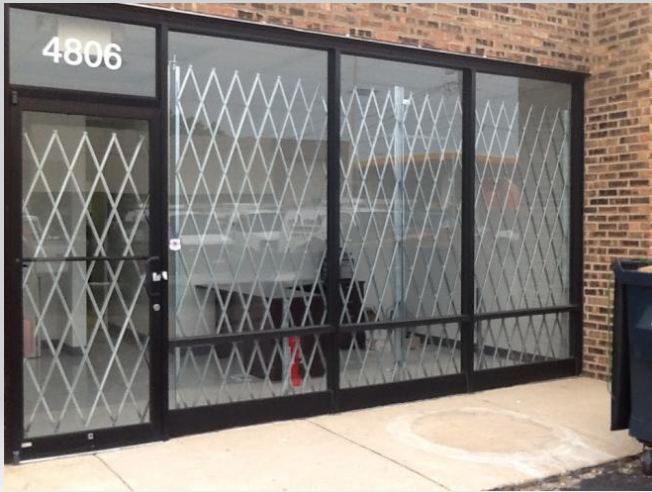
Pair Folding Gate / Galvanized Steel Store Front. For all gate configurations, there is a loss in height of about 6" as the gate is expanded. The stack width of a gate is approximately 1" to 2" per foot of travel.
